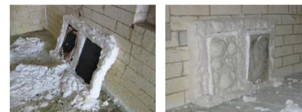
Failed primer test on panels shows the intumescent PFP coating has fallen away from the substrate
