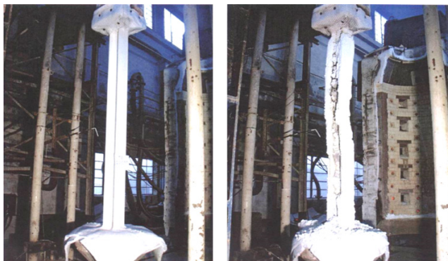
Loaded column before and after fire testing
