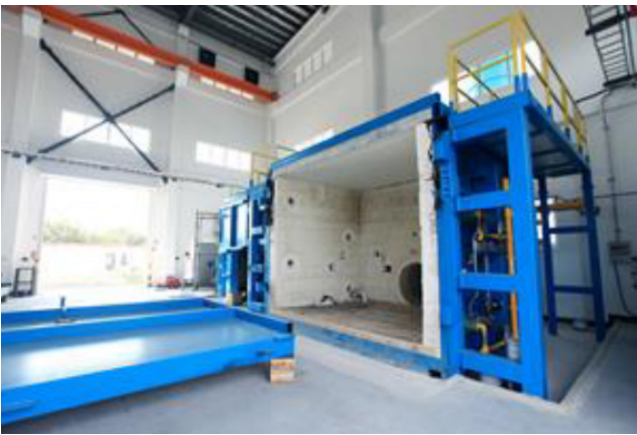
Fire testing furnace at PPG Global PFP Technology Center in Kunshan, China
